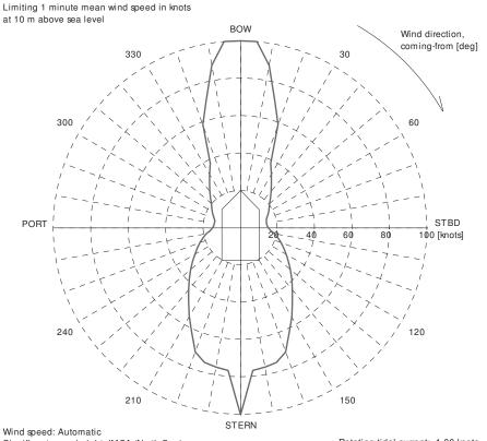
Wind speed: Automatic Significant wave height: IMCA (North Sea) Mean zero up-crossing period: IMCA (North Sea)
