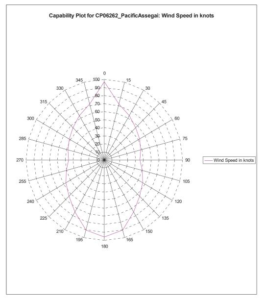
Wind Angle is stepped from 0 to 360 deg. Wave Angle is stepped from 0 to 360 deg. Current Angle is stepped from 0 to 360 deg. Wind Speed is Set Automatically. Wave Height is Derived from Wind Speed. Current Speed is 1.5 knots.
