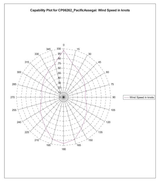
Wind Angle is stepped from 0 to 360 deg. Wave Angle is stepped from 0 to 360 deg. Current Angle is stepped from 0 to 360 deg. Wind Speed is Set Automatically.
