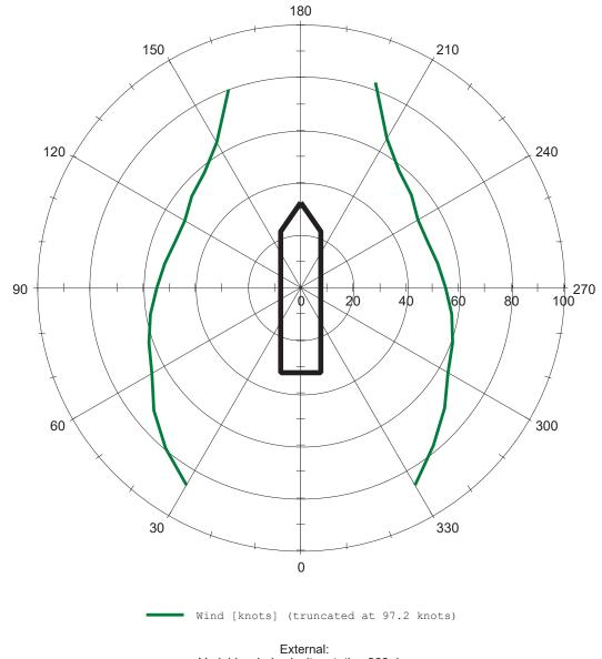
External: Variable wind velocity rotating 360 deg 1.50 knots wind generated current rotating 360 deg Variable wave height rotating 360 deg
